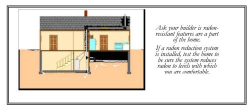
During the construction of a home, it is relatively easy to treat several foundations by connecting each area to a single vent, that may be concealed in walls. Plus, the system may be effective without the need to install and operate a fan.
